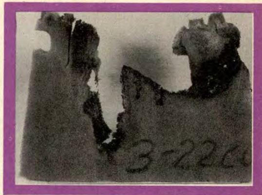
Side view of burned foam piece at fuel filler opening.
