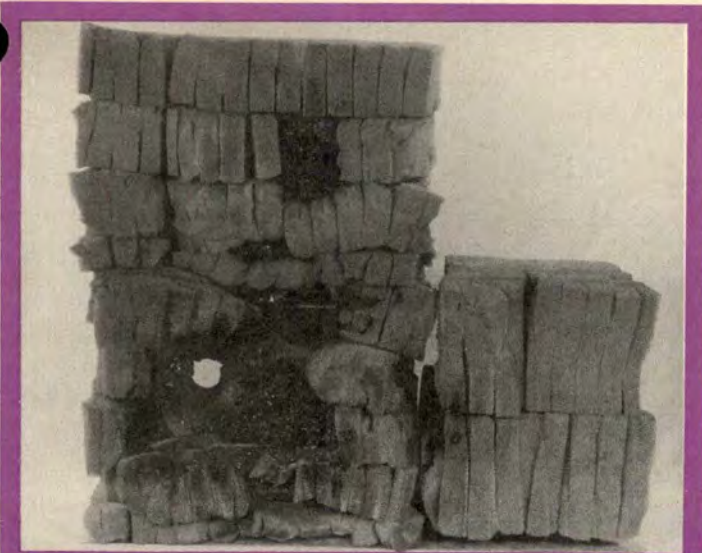
Overview of burned foam in the area of the Nr 3 main tank filler cap and dual level control valves.
